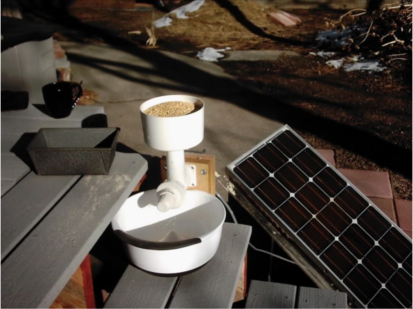
caption: MODIFIED GRAIN GRINDER WORKING OFF A SMALL PV PANEL. GOOD FOR A LOAF AN HOUR ON SLOW SPEED.
