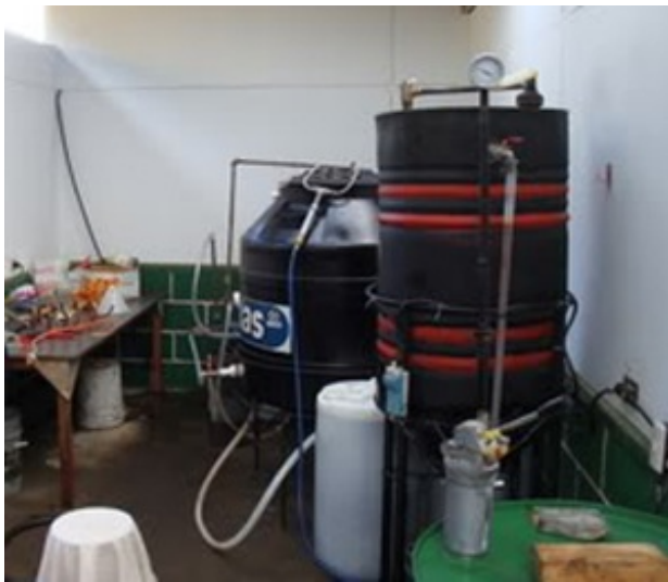
[Image 1] A local scale biodiesel processing set-up in Costa Rica.
